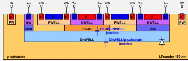
Cross-section of the HV-CMOS pixel
