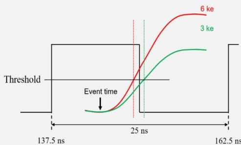
Detection of the hit time for different energies at the edge of the clock
