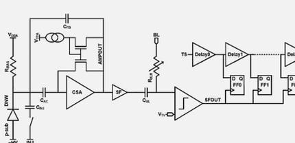
Pixel readout modified for the TDC method
