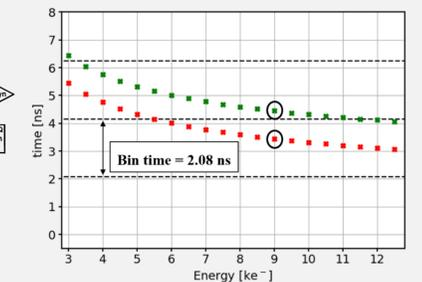
Time-stamp for different signal heights and particle detection times
