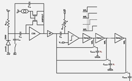
Pixel readout for the analog sampling method
