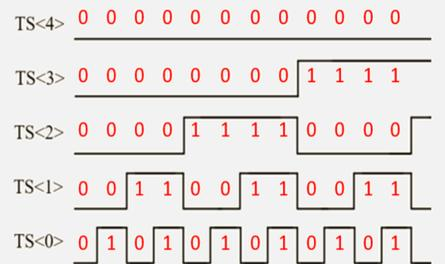
Timing diagram of the time-stamp bits. For simplicity, only the 5 Less Significant Bit are shown
