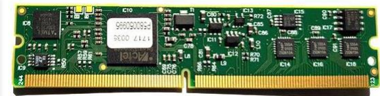
IPMC mezzanine board
