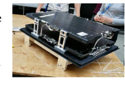
The detector (left) was built in 2018 and consists of 2 scintillation layers of 60x40 cm (4 tiles/layer), 2 SiPM per tile, for a total of 16 channels
