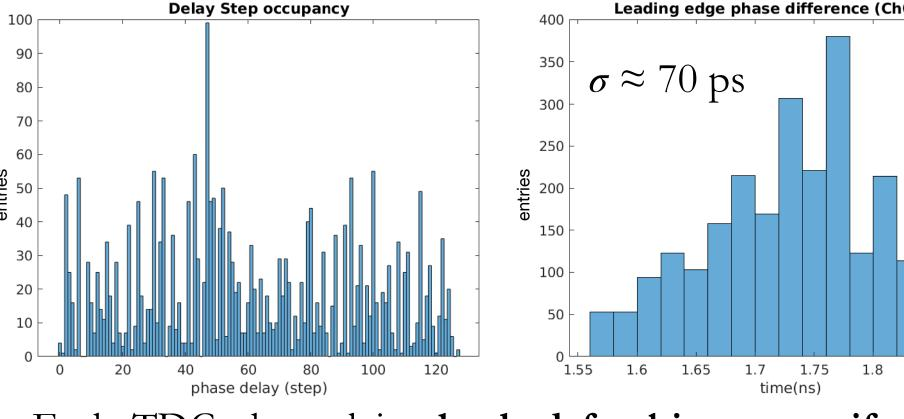
Each TDC channel is checked for bin non-uniformity (left). The resolution can be obtained by sending the same pulse to each channel and measuring the phase difference between every pair (right) which is the square sum of the single channel resolution. Therefore, channel resolution can be calculated by solving linear systems and typical achieved values range from 40 to 90 ps.
