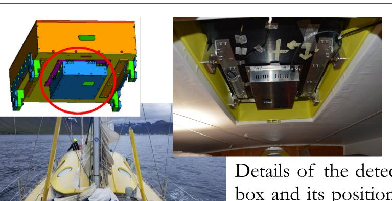
Details of the detector box and its positioning into the sailboat (electronics into the aluminum box)
