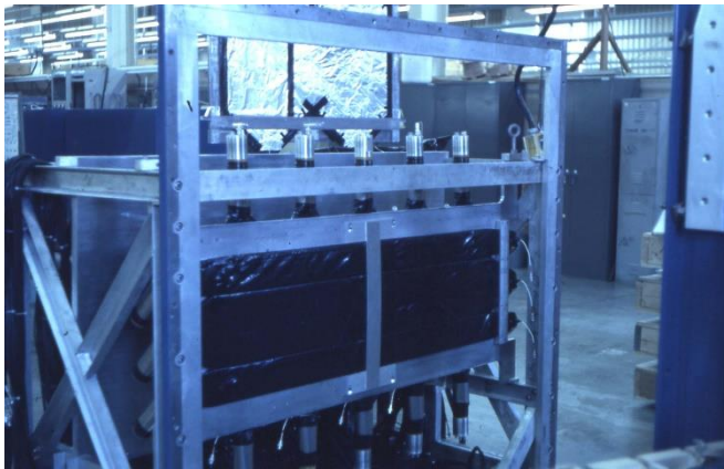
8 GeV Spectrometer – “ \pi -e separator” i.e. EM Calorimeter Designed long before EGS or GEANT shower Monte Carlos
