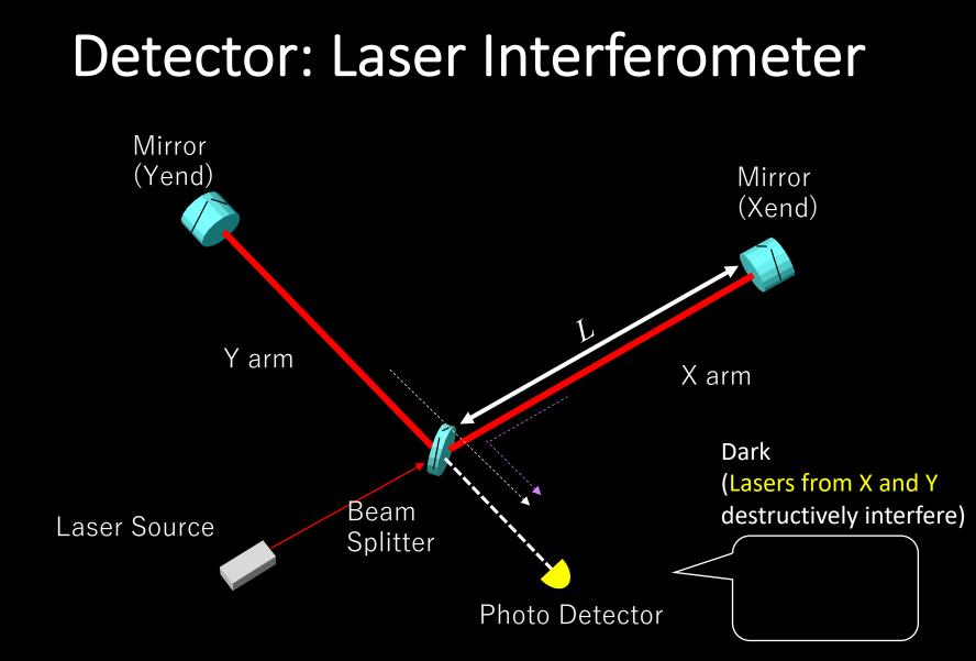
Optical sensor detecting the length difference between X and Y arms
