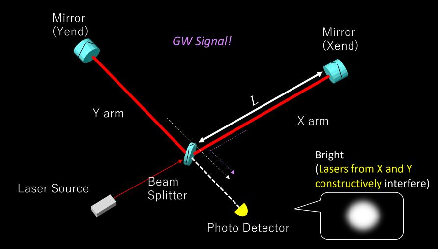
Optical sensor detecting the length difference between X and Y arms
