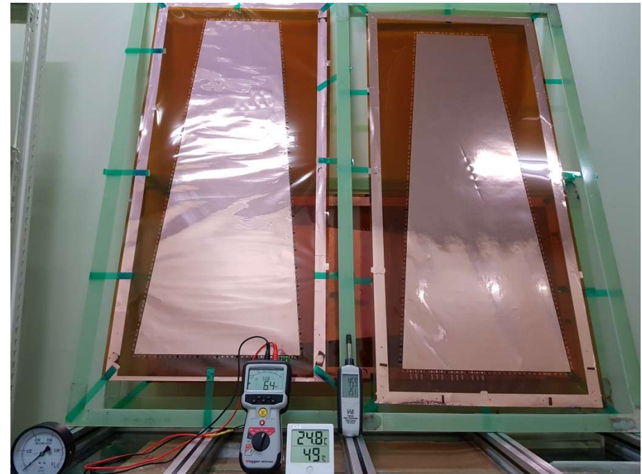
Leakage current measurement
