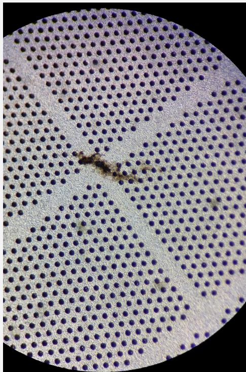
The damages done by a spark.
