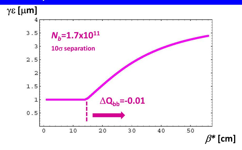
emittance for the low-emittance scheme determined by  $\Delta Q$
