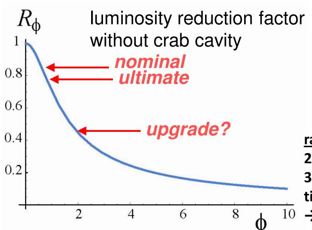
effective beam size  $\sigma \rightarrow \sigma / R_{\phi}$
