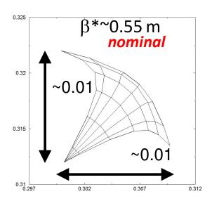
nominal tune footprint up to  $6\sigma$  with 4 IPs & nom. intensity  $N_b=1.15\times10^{11}$  $I=10^{34}$  cm<sup>-2</sup>s<sup>-1</sup>
