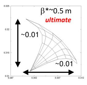
tune footprint up to  $6\sigma$  with 2 IPs at ultimate intensity  $N_b$ =1.7x10<sup>11</sup> L=2.3x10<sup>34</sup> cm<sup>-2</sup>s<sup>-1</sup>
