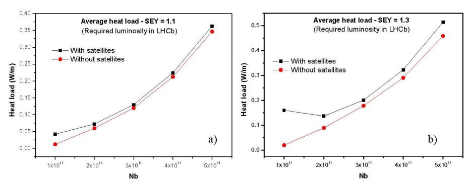
satellite intensity is varied as the inverse of main-bunch intensity to yield target luminosity of 2x10<sup>33</sup> cm<sup>-2</sup>s<sup>-1</sup> in (S)LHCb
