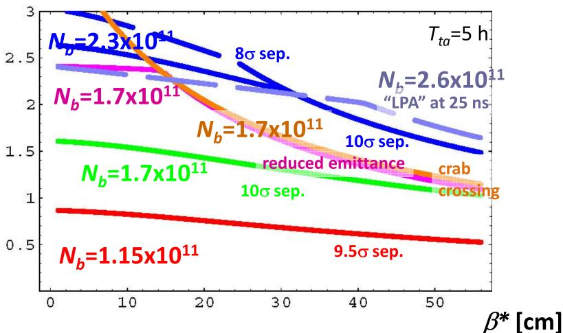
beam intensity is much more important than  $\beta^*$ , reducing  $\beta^*$  only helps with crab cavities or with smaller emittance
