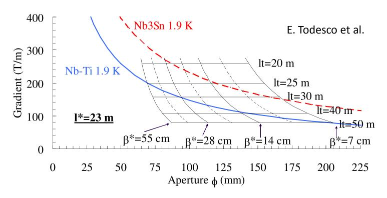
This was the base to explore a wide parameter range also with Nb-Ti Confirming (and correcting) the first results of F. Ruggiero et al. (Epac04) showing that there was room for a first upgrade with Nb-Ti.
