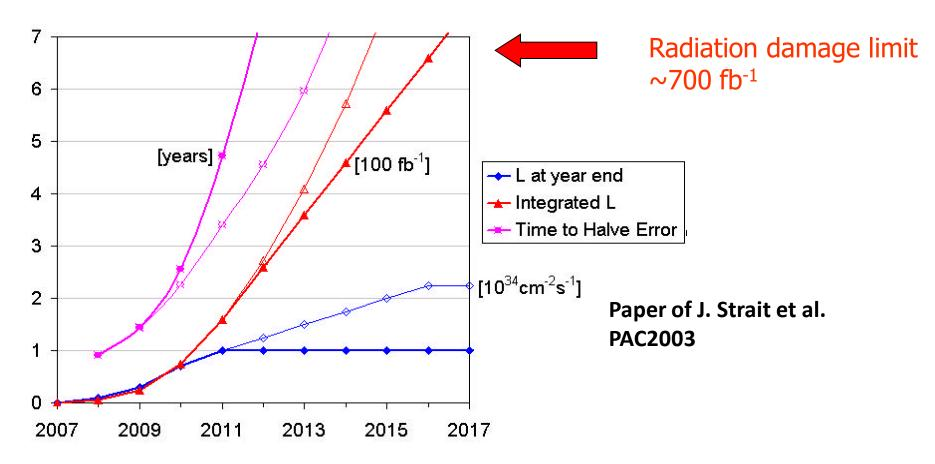
**Beam commissioning 2007** – full luminosity in 4 years – ultimate luminosity in 5 years Needs of stronger triplet  $\Rightarrow$  Nb3Sn technology  $\Rightarrow$  LARP (US program for LHC)
