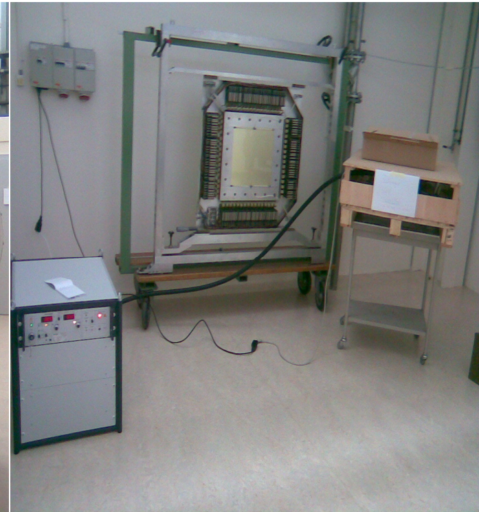
High voltage (100 kV) system Under test
