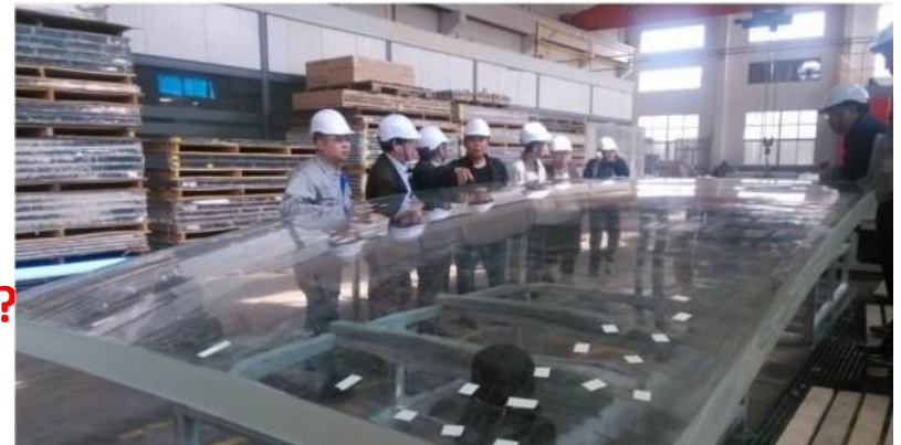
Thermoforming the spherical panel: 3m x 8m x 120mm
