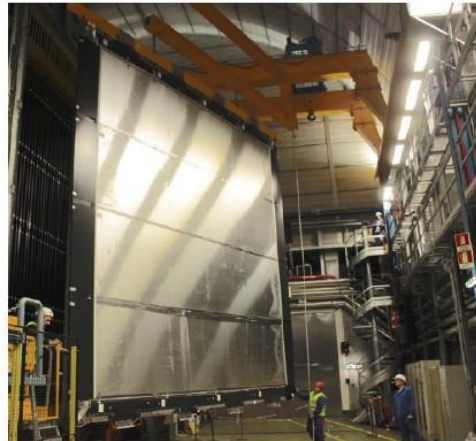
Fig. 3. Schematic view of a plastic scintillator strip wall. Prague, October 24, 2019
