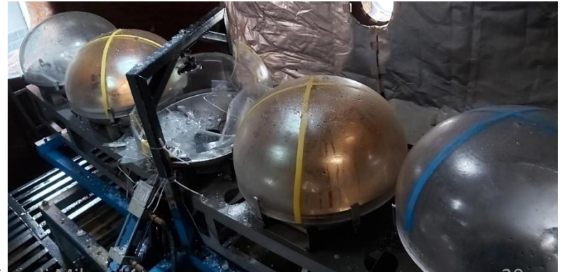
Implosion test with a PMT module
