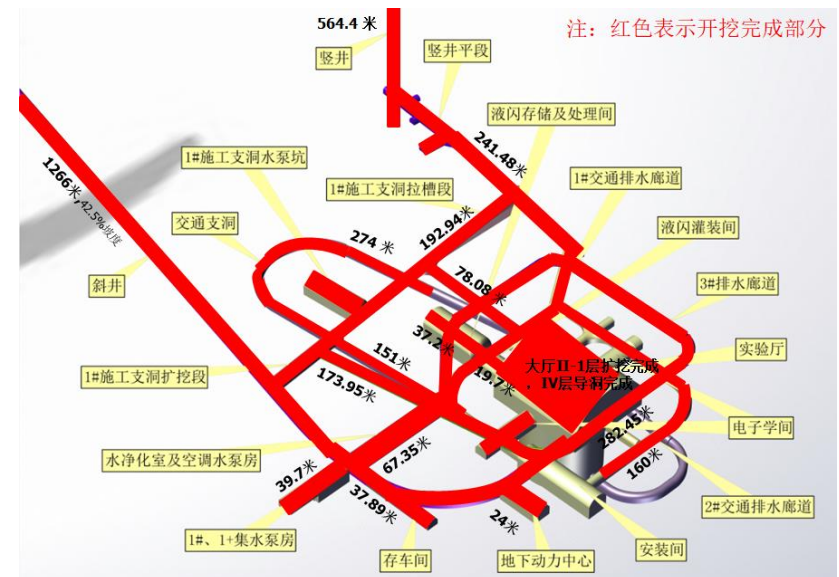
Status of the underground civil construction
