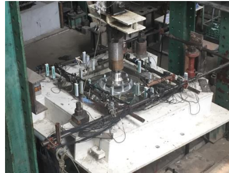
Batch test of acrylic node
