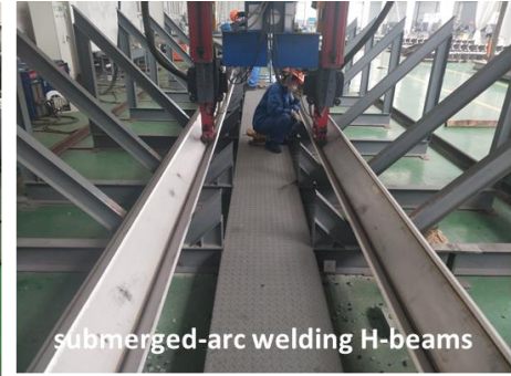
Deep-melting bottom welding
