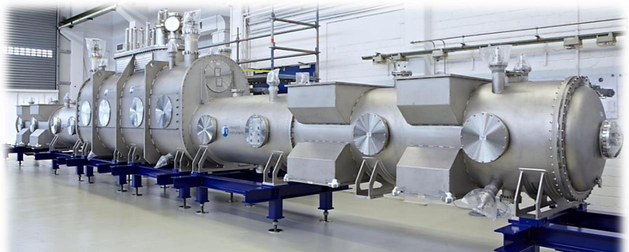
**Windowless Gaseous Tritium Source cryostat**
