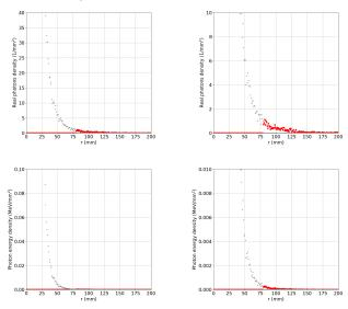
Flat screen perpendicular to z axis (of propagation) @ 1.0 m from IP Real photons at radius > 0.0795 m (in red): 38340.0 Real photons 0.13 m < radius < 0.14 m : 1840.0 Total energy photons at radius > 0.0795 (in red): 8.828809359632407 MeV Real photons 0.13 m < radius < 0.14 m : 0.3069129984266657 MeV
