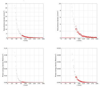
Flat screen perpendicular to z axis (of propagation) @ 1.4000000000000001 m from IP Real photons at radius > 0.0795 m (in red): 99360.0 Real photons 0.13 m < radius < 0.14 m: 5540.0 Total energy photons at radius > 0.0795 (in red): 44.91407643539817 MeV Real photons 0.13 m < radius < 0.14 m: 1.58614008540713668 MeV
