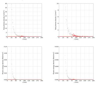
Flat screen perpendicular to z axis (of propagation) @ 0.8 m from IP Real photons at radius > 0.0795 m (in red): 20540.0 Real photons 0.13 m < radius < 0.14 m: 940.0 Total energy photons at radius > 0.0795 (in red): 2.9515396243735132 MeV Real photons 0.13 m < radius < 0.14 m: 0.10260858924469583 MeV
