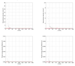
Flat screen perpendicular to z axis (of propagation) @ 0.4 m from IP Real photons at radius > 0.0795 m (in red): 3000.0 Real photons 0.13 m < radius < 0.14 m: 100.0 Total energy photons at radius > 0.0795 (in red): 0.1044432955091591 MeV Real photons 0.13 m < radius < 0.14 m: 0.0030197209270645606 MeV
