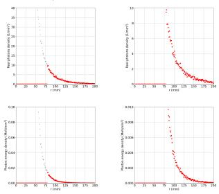
Flat screen perpendicular to z axis (of propagation) @ 2.0 m from IP Real photons at radius > 0.0795 m (in red): 264380.0 Real photons 0.1.3 m < radius < 0.14 m : 14280.0 Total energy photons at radius > 0.0795 (in red): 243.07789423378566 MeV Real photons 0.13 m < radius < 0.14 m : 9.49258094856397 MeV
