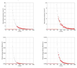
Flat screen perpendicular to z axis (of propagation) @ 1.6 m from IP Real photons at radius > 0.0795 m (in red): 143160.0 Real photons 0.13 m < radius < 0.14 m : 7900.0 Total energy photons at radius > 0.0795 (in red): 84.44894511198567 MeV Real photons 0.13 m < radius < 0.14 m : 3.364563405568128 MeV
