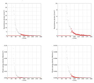
Flat screen perpendicular to z axis (of propagation) @ 1.2000000000000000 m from IP Real photons at radius > 0.0795 m (in red): 64860.0 Real photons 0.13 m < radius < 0.14 m: 3400.0 Total energy photons at radius > 0.0795 (in red): 21.35066246857667 MeV Real photons 0.13 m < radius < 0.14 m: 0.7442226887110909 MeV
