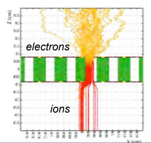
left: electron avalanche simulation of a single stage LEM (Garfield)
