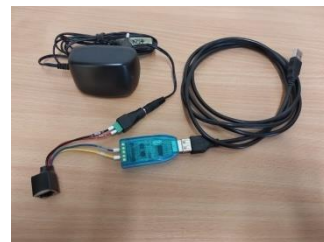
RS-485 Bus signals and power (+12V)
