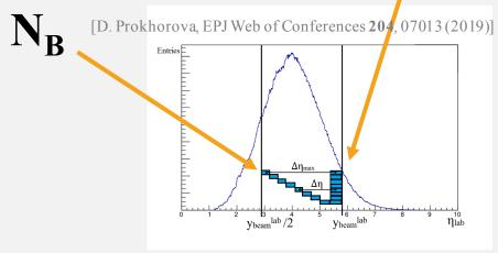
uncorrected rapidity distribution of all charged hadrons produced in p + p @158 GeV/c in NA61/SHINE experimental acceptance
