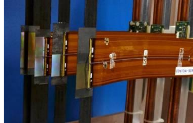
Mimosa-26 sensors mounted on extra-lightweight CF cooling panels
