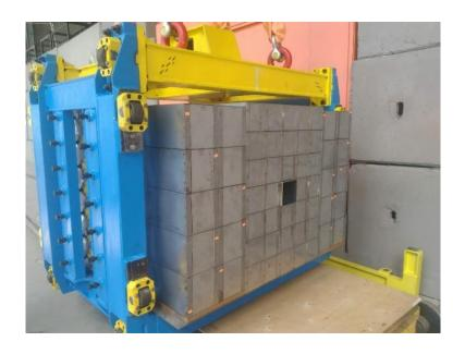
CBM Calorimeter modules setup for usage at BM@N
