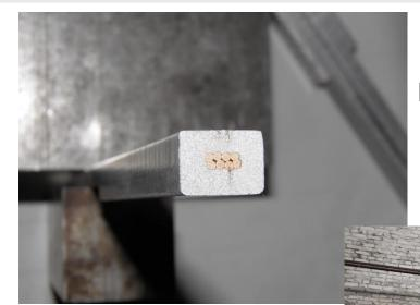
Extrusion test for SC cable prototype
