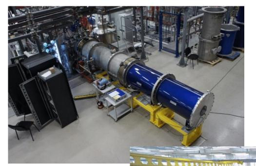
SIS100 quadrupole unit mounted in the test cryostat (blue) at JINR, Dubna
