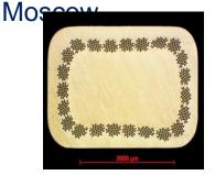
Photo of the cross section of the superconducting cable
