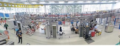
Test facility for superconducting magnets at JINR
