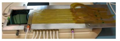
Jig for sensor bonding
