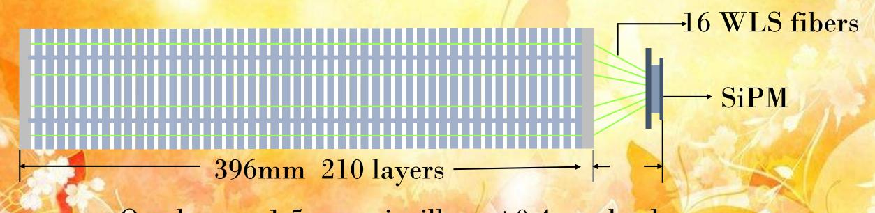
One layer: 1.5mm scintillator+0.4mm lead
