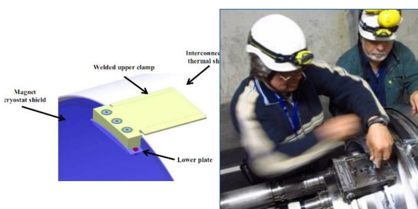
New thermal shield design, removing the necessity of grinding
