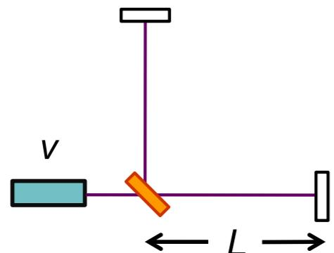
**Laser interferometry (cavities)**
