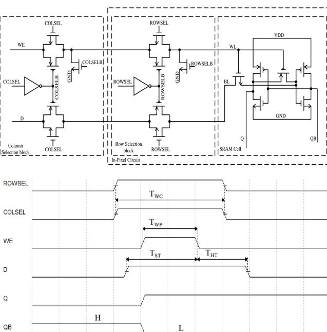
The schematic of the configuration cell for pixel detectors is composed of a column selection block, a row selection block and a SRAM cell.
