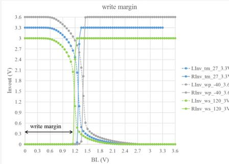
A minimum bit line voltage required to flip the state of the SRAM cell is called write margin. It is used to measure the ability to write data into the SRAM cell. The minimum write margin is about 1.15V.
