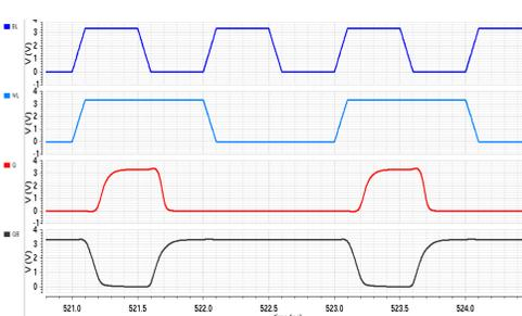
According to the write waveform, the outputs of both Q and QB depend on the BL signal. When the WL signal is at high level voltage, the output Q follows the BL signal with a delay of 137 ps from "1" to "0" and 184 ps from "0" to "1". When the WL signal is at low level voltage, the outputs Q and QB is kept its previous value, respectively.
