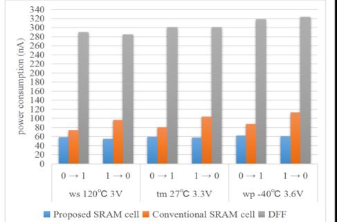
Compared to the conventional SRAM cell and DFF, the power consumption of the proposed SRAM cell is reduced by 20% and 80% during the rising edge, respectively, and is decreased by 43% and 81% during the falling edge, respectively.
