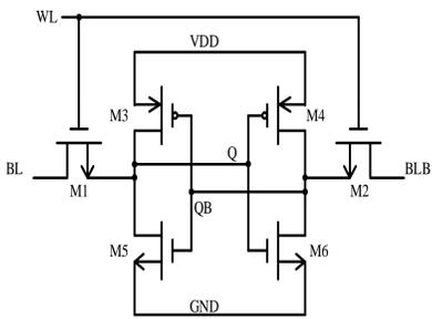
The conventional 6T SRAM cell is composed of two cross-coupled inverters (M3~M6) and two access transistors (M1, M2). There are three operating modes in SRAM, write, read and hold.
