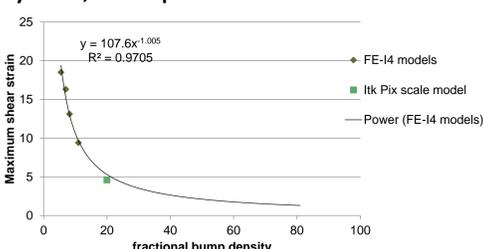
A plot of shear strain for FEI4 models vs bump fractional volume produces the fit shown right. A full ITk pix scale device with 25µm of copper sits nicely on this curve.
