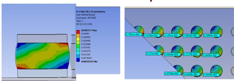
These plots from FEA show the shear strain for an ITk Pix scale device. FEI4 models gave calculated cycles to failure of a few 10s of cycles, comparable to the data shown above.
