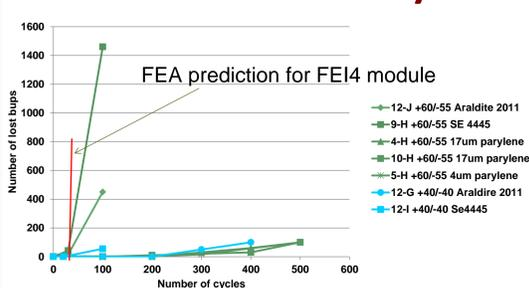
Further mitigation of the thermal stress in the BB layer comes from parylene coating which is the baseline for HV protection. This plot shows even FEI4 modules with thick
