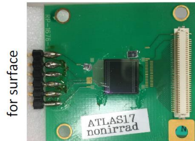
Sample on PCB (wirebonded)
