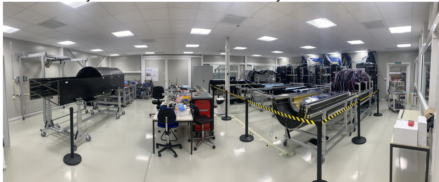
Half-Barrel Assembly (a hierarchical Russian doll like assembly) All half-layers are first tested individually.
