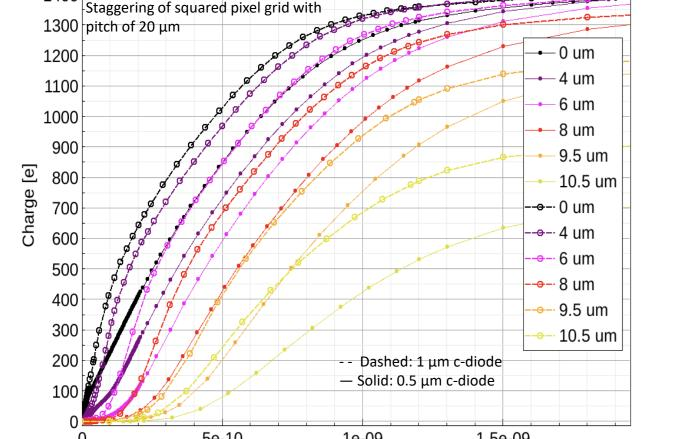
1.5e-09 → Trade-off: Time [s] Small collection electrode → Small capacitance but lower field Large collection electrode -> Large capacitance but higher field
