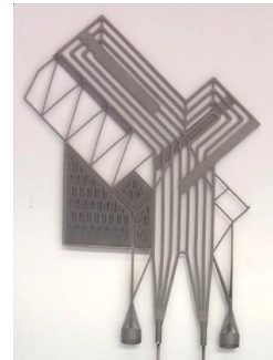
3d printed Titanium substrates, already prototyped for Upgrade I
