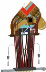
wire bonding and HV/LV/data cable attachment
