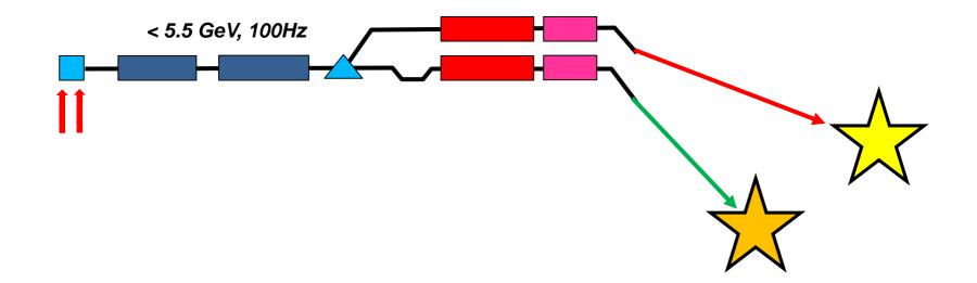
FEL-1/FEL-2 producing independent pulses for two experiments at up to 16keV @ 100 Hz
