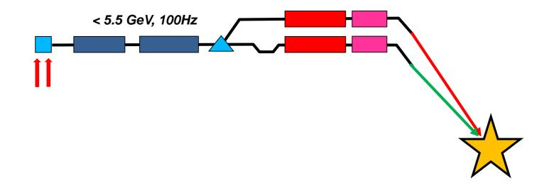
FEL-1/FEL-2 producing independent pulses for one experiment at up to 16keV @ 100Hz
