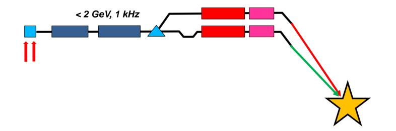
FEL-1/FEL-2 producing independent pulses for one experiment at up to 2keV @ 1 kHz
