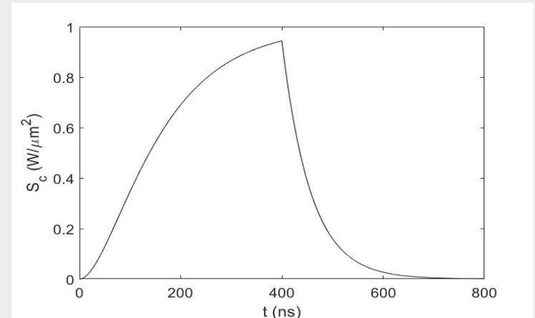
Maximum amplitude of the modified Poynting vector as a function of time
