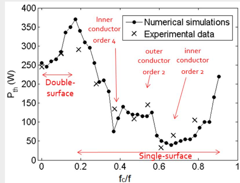
Multipactor RF power threshold as a function of the ratio between the cyclotron frequency and the RF frequency. For a coaxial line at  $f = 1.145 \text{ GHz}$
