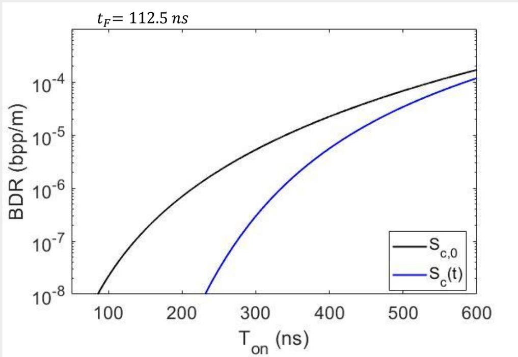
BDR as a function of the time that the generator is on, for the RF gun operating with 200 MV/m at cathode
