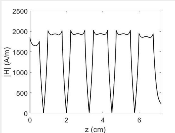
Magnetic field at the gun surfaces as a function of the axial position for 1 MV/m at cathode
