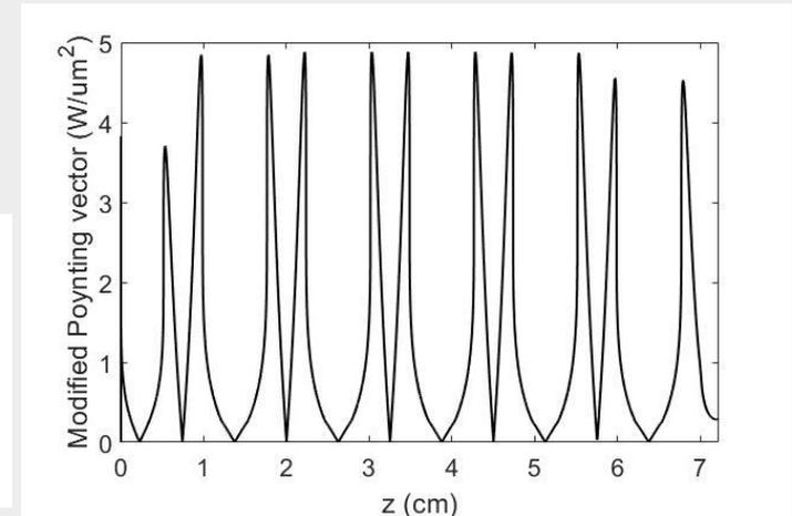
According to ref. (1), a value of  $S_c = 5 \text{ W}/\mu\text{m}^2$  for a pulse length of 200 ns gives a breakdown rate of  $BDR = 10^{-6} \text{ bpp/m}$ . Using this data, the constant can be evaluated  $C = 9.765625 \times 10^{27} \text{ W}^{15} \cdot \text{ns}^5 \cdot \text{m} \cdot \mu\text{m}^{-7.5} \text{ bpp}^{-1}$
