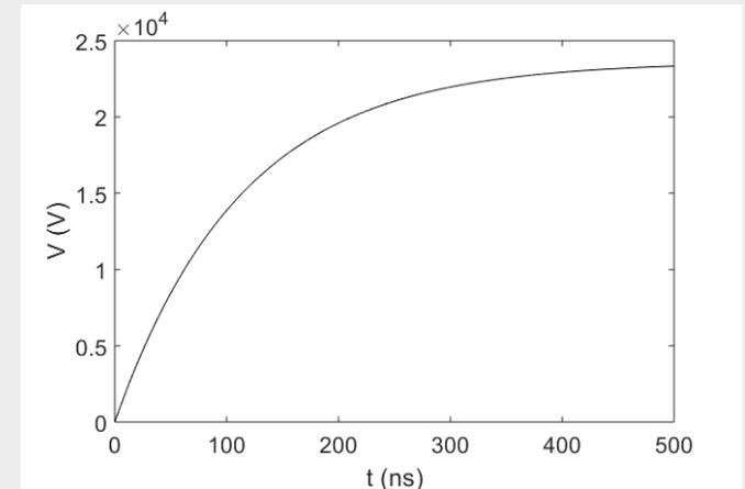
Coaxial voltage amplitude during the cavity filling
