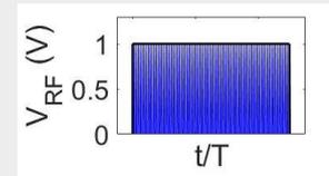
For the RF gun  $\longrightarrow$   $S_c(t) = \begin{cases} S_{c,0} (1 - e^{-t/t_F})^2, & 0 \leq t \leq T_{on} \\ S_{c,0} (1 - e^{-T_{on}/t_F})^2 e^{-\frac{2(t-T_{on})}{t_F}}, & t \geq T_{on} \end{cases}$
