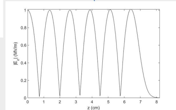
RF electric field along the gun only for  $\pi$ -mode
