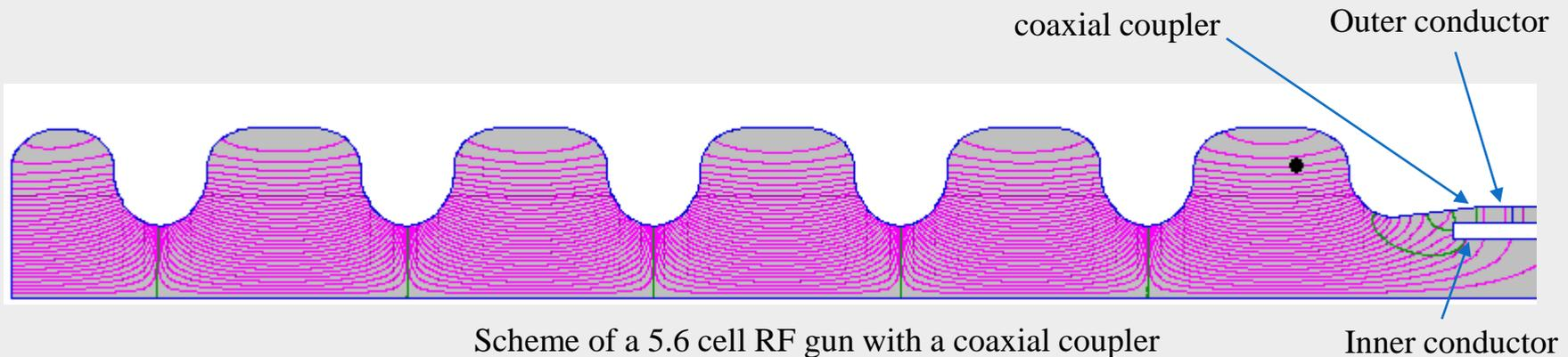
Scheme of a 5.6 cell RF gun with a coaxial coupler
