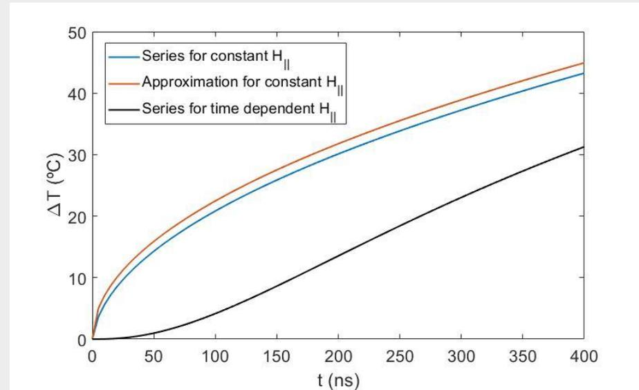
Maximum temperature increase in the RF gun as a function of time
