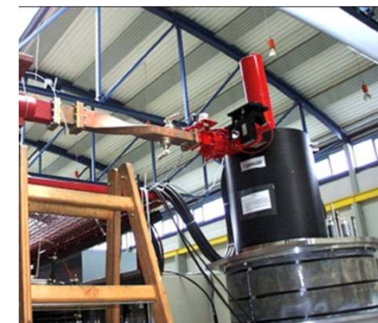
TH2100 klystron at PSI
