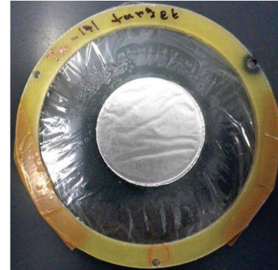
Figure 7: The final arrangement of the ^{171}\text{Tm} target provided to n_TOF CERN.
