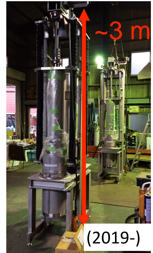
High precision piston for emulsion gel production
