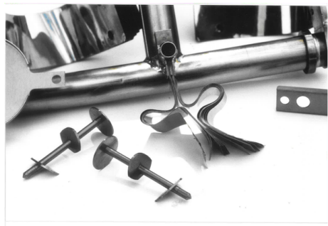
Figure 9: Tantalum container used at ISOLDE for a static molten lanthanum target. The external diameter is 21 mm. A tantalum ring for reinforcement at the beam window in case of shocks induced by the pulsed PSB beam can be seen on the right, while baffles to prevent release of metal from the target into the ion source through the chimney are seen in front
