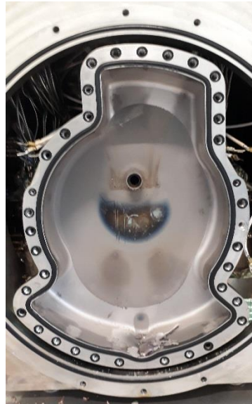
Figure.34: Pictures of ion source vacuum vessel and the line connection underneath the source
