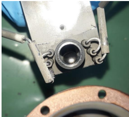
Figure.35: Picture of the transfer line filled with solid LBE
