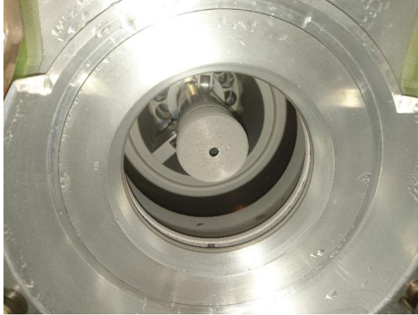
Figure.32: Extraction electrode coated with LBE
