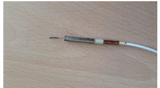
Figure 14: Heating element 4 broken.
