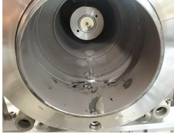
Figure.33: Macroscopic quantities of LBE underneath the ion source
