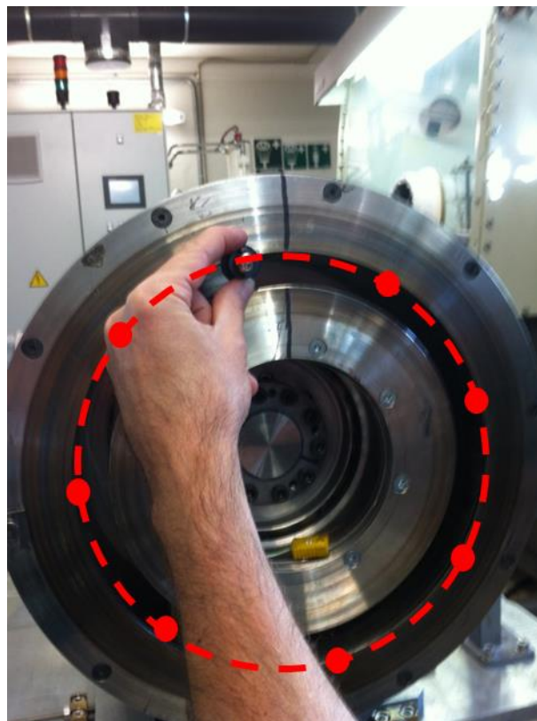
Figure5: Outer Pump assembly measured in static position.
