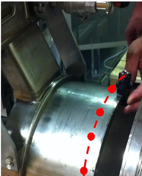
Figure 3: Survey target and adapter used to measure front cylinder plane.
