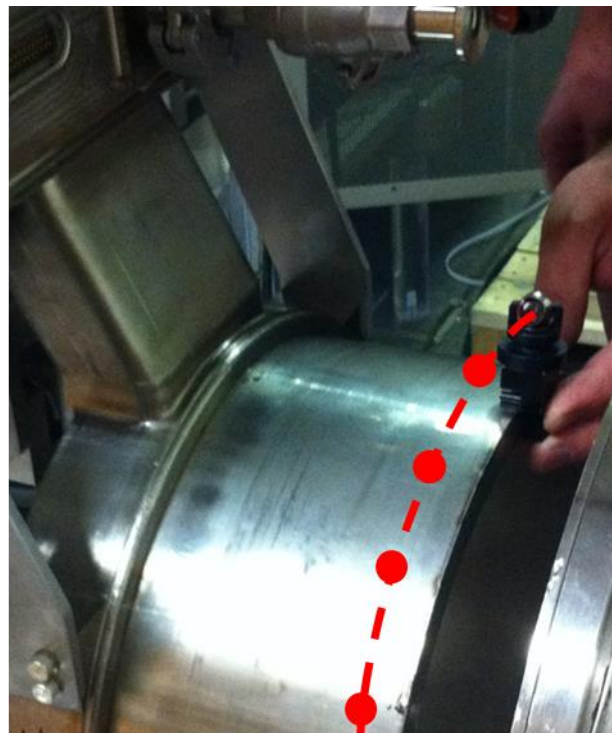
Figure 8: Survey target and adapter used to measure front plane cylinder.
