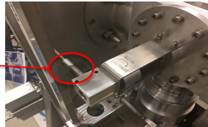
Position of screws to tight (Offline 2 picture)
