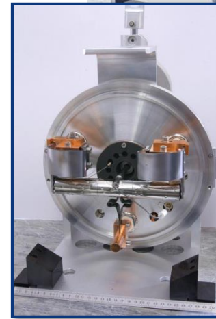
Standard ISOLDE target unit – without double enclosure
