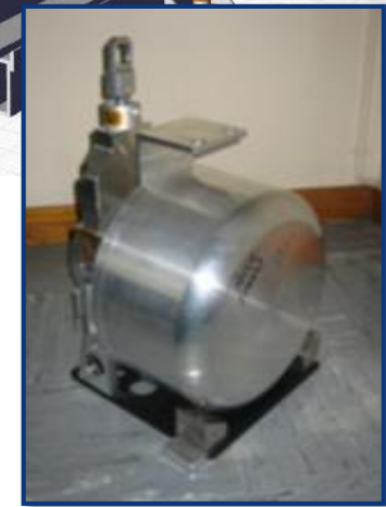
Standard ISOLDE target unit – with double enclosure
