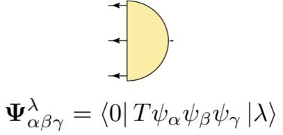
**Spectral decomposition**: extract gauge-invariant baryon poles from gauged-fixed quark n-point functions.
