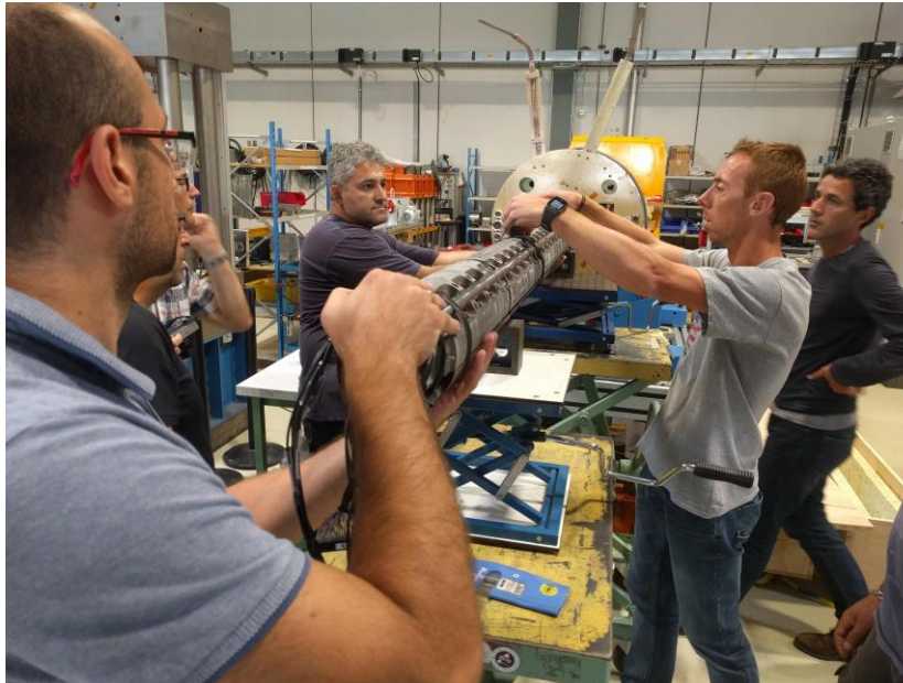
Beam screen insertion in short model [P. Ferracin, J. C. Perez, et al.]
