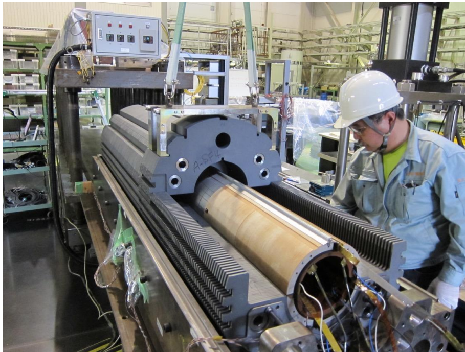
Collaring with iron [T. Nakamoto, M. Sugano, et al.]
