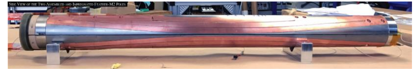
Feather 2.3-4 HTS Insert (Courtesy of G. Kirby and J. van Nugteren, CERN)
