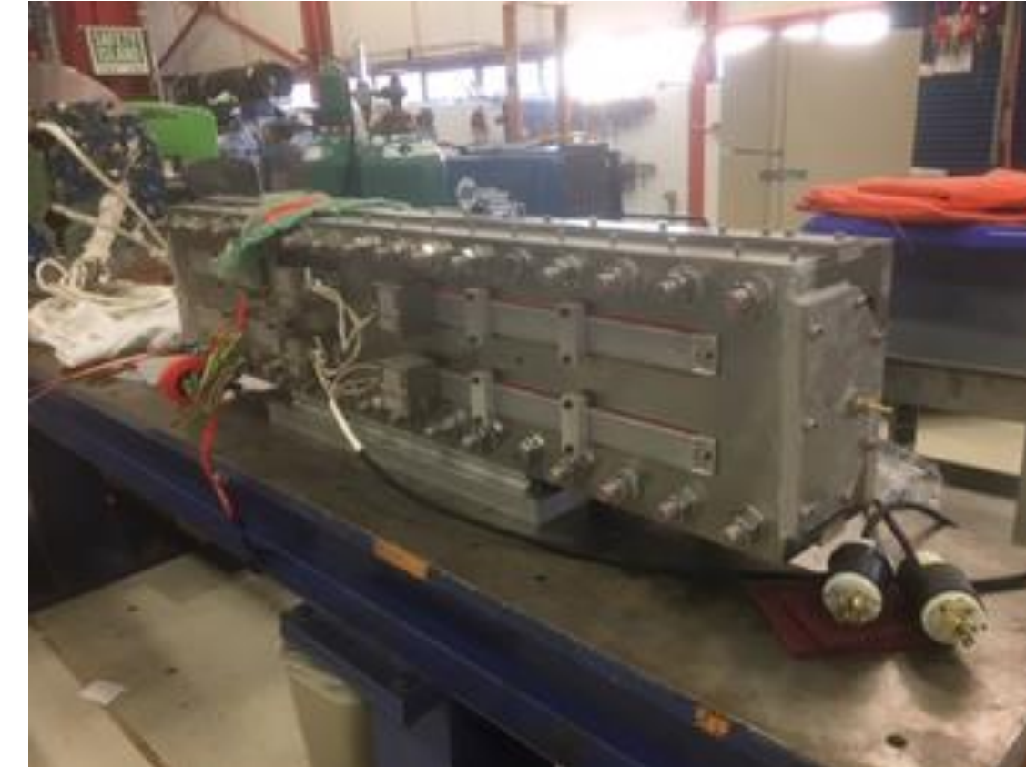
Coil lead splicing, epoxy impregnation
