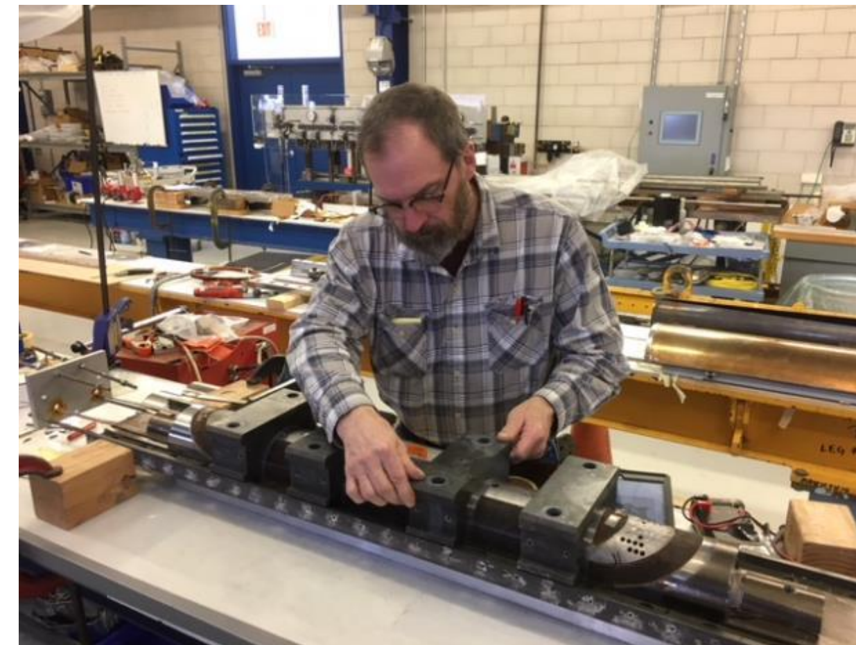
Coil lead splicing, epoxy impregnation
