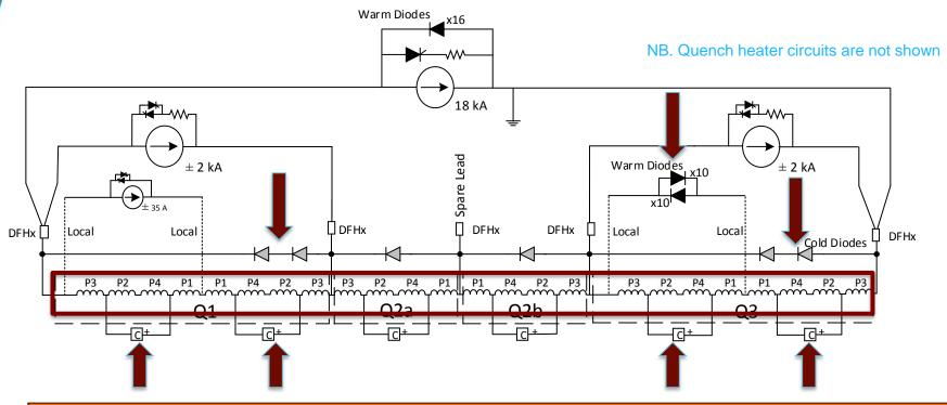
The **quench protection strategy** for the inner triplet of the HL-LHC is such that any quench in a superconducting element of the circuit will trigger the quench protection of all the elements of the circuit (switching off all the power converters, firing quench heaters and CLIQ units in all magnets).
