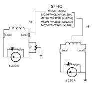
The proposal is to use the LHC design - and associated integration strategy - for feeding the HL-LHC corrector circuits rated at DC current of 200 A and below. The circuits concerned are: MQSXF, MCSXF/MCSSXF, MCOXF/MCOSXF, MCDXF/MCDSXF and MCTXF/MCTSXF
