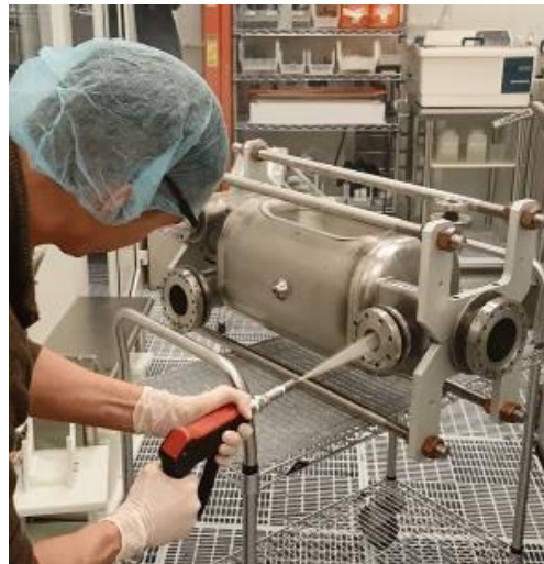
RFD HPR and Cleanroom Assembly (ANL/FNAL facility)
