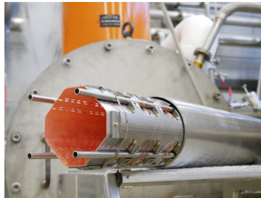
80 cm long Beam screen prototype at HL-LHC beam screen test stand
