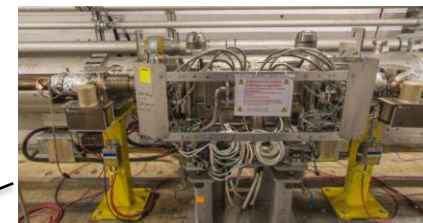
TCLIB: auxiliary protection collimator
