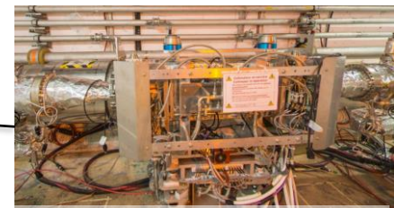
TCLIA: auxiliary protection collimator
