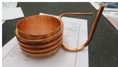
1st prototype: significant voids in brazing
