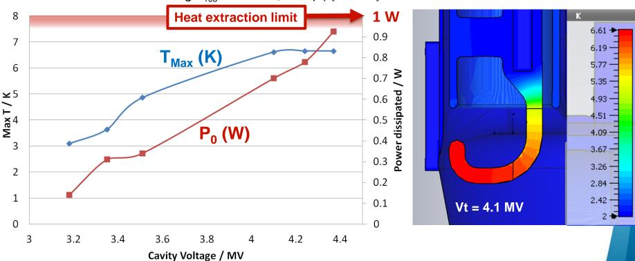
From CST simulations using  $R_{res} = 5 \text{ nOhm}$ , K = f(T) [G. Burt]
