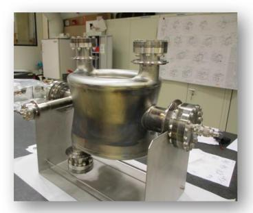
All the cavities following **BCP-based** standard **surface treatment** procedure: bulk BCP, 10h 600C, light BCP, HPR, 24h 120C. 9th HL-LHC Coll. Meeting | Fermilab | 15 Oct. 2019 | Silvia Verdú-Andrés
