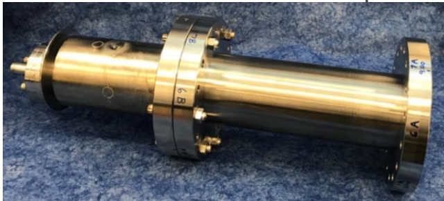
Test box can with HHOM coupler
