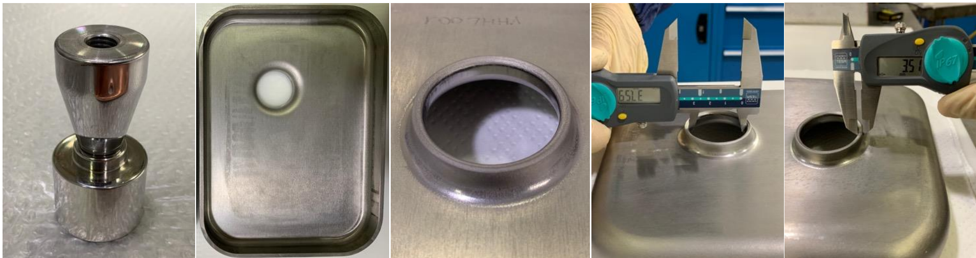
From Left: Extrusion Tool. V-HOM Results. Results: nominal \text{\O}37.63\text{mm} , nominal thickness 2.2mm!
